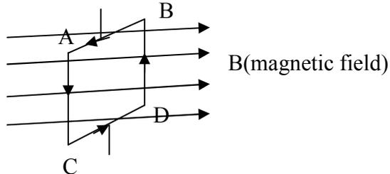
Here the conductors AC and BD are perpendicular to the field. A current I is passed through the loop.
